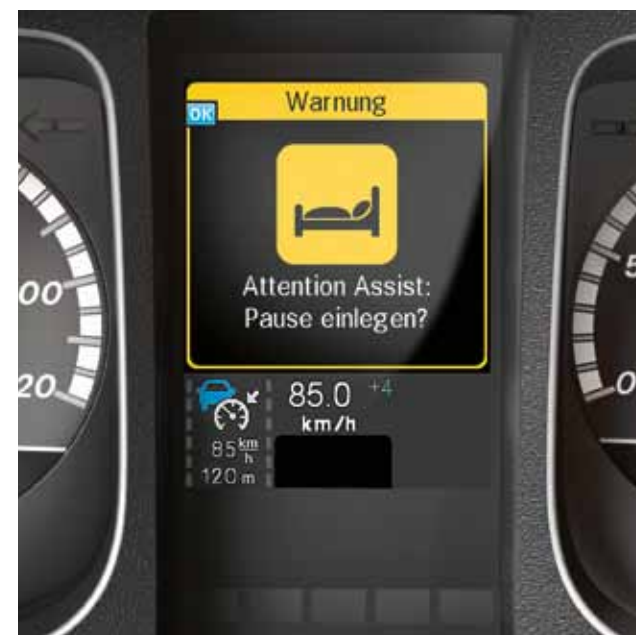
Attention Assist 3) . The system can recognise increasing tiredness and recommend the driver takes a break.
