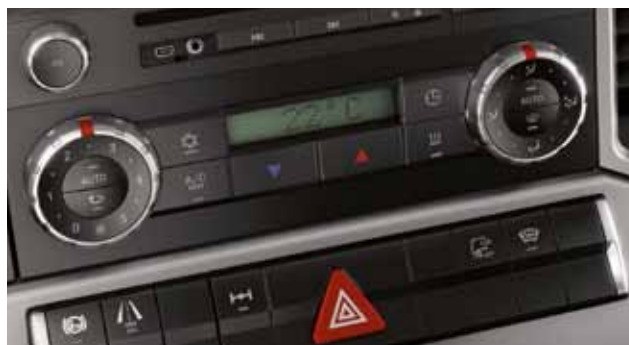
Automatic climate control 2) . The system automatically adjusts the air volume, distribution and temperature in line with the ambient conditions and offers additional comfort and convenience functions.
